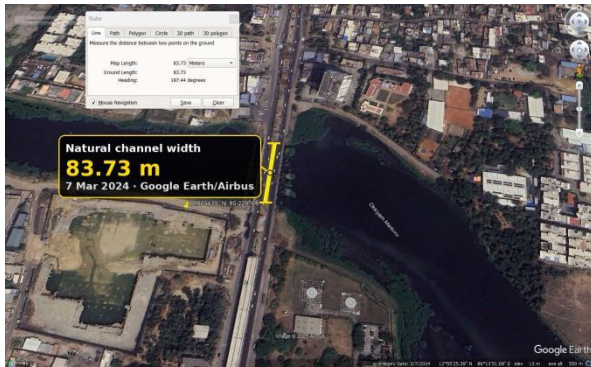
Fig 5 — Before: Okkiyam Maduvu, March 2024. Pre-construction channel width: 83.73 m. Imagery: © 2024 Airbus / Google Earth.
